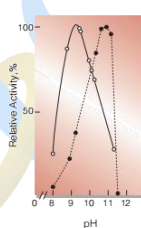
Fig.3. pH-Activity ○ α-KIC → Leu in 1M ammonium buffer ● Leu → α-KIC in 0.2M glycine- KOH buffer
